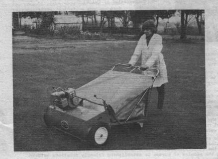
The above illustration shows just one of our comprehensive range of turf management products. Illustrated is the HORWOOL 36" Power Sweep, powered by a 3 h.p. 4-stroke engine. The separate clutch system allows high manoeuverability for the eight long-life nylon brushes to sweep clean in the smallest of areas. This model is available in two sizes: 25" and 36" sweeping widths.
